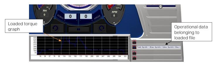
The loaded graph will appear in the graph window and torque-position ranges will be adjusted accordingly. Operational data for the loaded graph appears in the side window.
