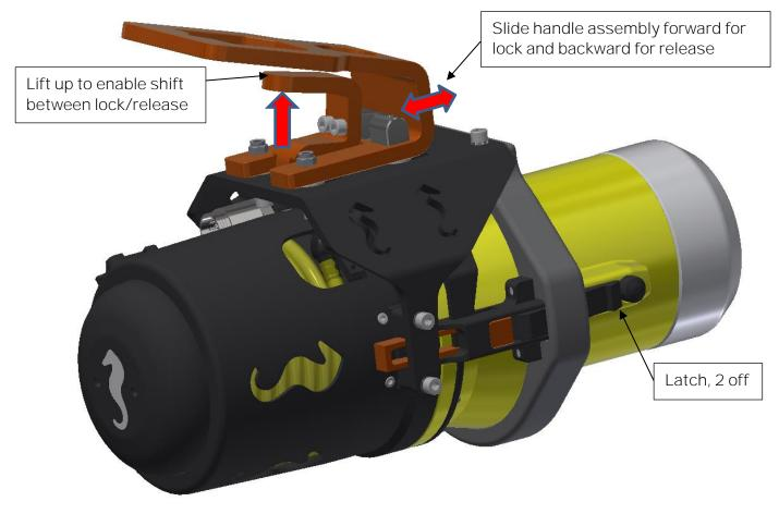
Figure 8, Latch mechanism
