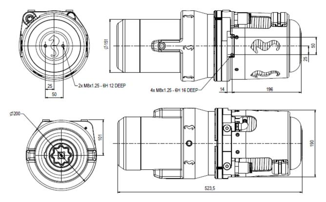
Figure 11 LWETT AUV configuration - main dimensions and bolting interface
