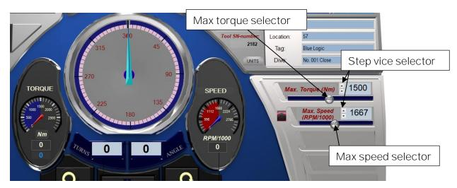
Adjustment can be performed by pressing and dragging the slider handles in the Operation Set Limit Board, or by clicking the one-step vice selector. Values can also be typed directly in the Operation Set Limit Board.
